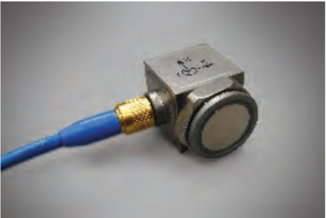
Four, 3-axis accelerometers are fixed to the corners of oscillating frame.
