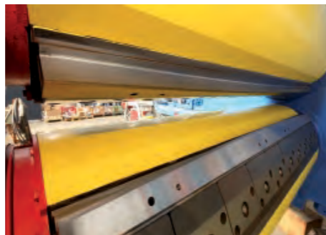
Danieli DanCut knives on a drum shear. All DanCut shear blades are made in tough, hardened tool steel and allow multiple resharpenings up to the minimum resisting section of the blade.
