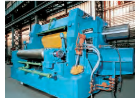
Compact and sturdy drum shear with cassette design.
