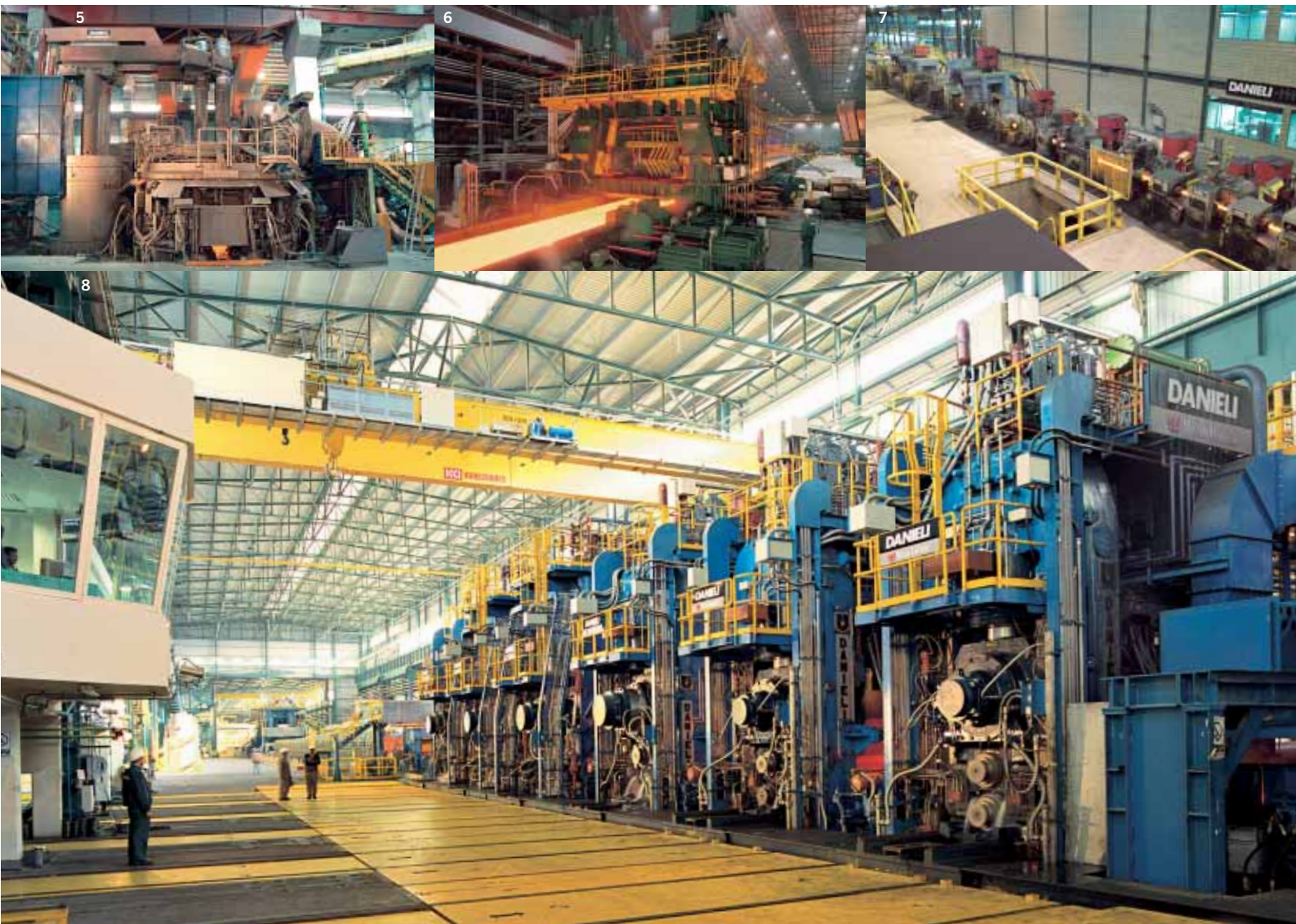
5 185-t AC Danarc EAF equipped with Module technology.
