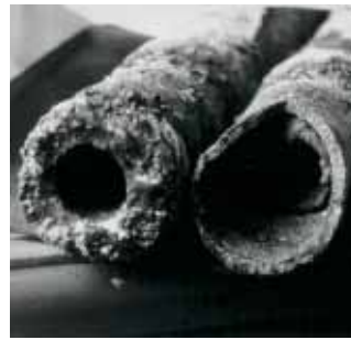
12 SEN-Submerged Entry Nozzle wear that was believed to be due to M-EMS was in fact due to insufficient SEN immersion depth.
