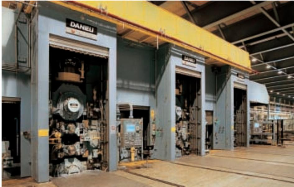
equipped by only one shapemeter and constituted of five stands, where the last one is of six-high type.
